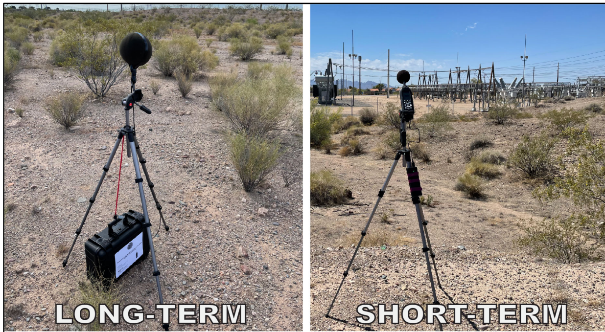
Figure 4-1. Examples of Long-Term and Short-Term Noise Measurement Setups
